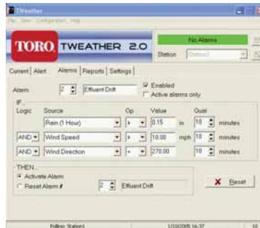
When using SitePro's ET-based programming capability, the optional T.Weather software module employs the "if/then" statements of our WeatherLogic feature, allowing your system to react to real-time weather conditions. This allows you to establish an interactive link between the weather station and the SitePro central control system.
