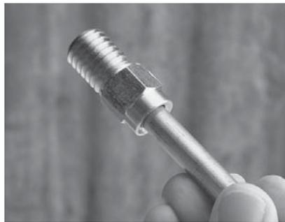
2. Screw the lever into the recessed female thread of the adaptor with a spanner:
