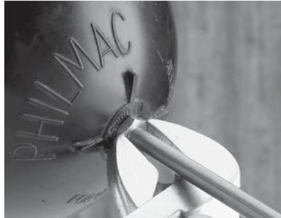
2. For  $\frac{3}{4}$ ", 1" and  $1\frac{1}{4}$ " valves tighten the nut against the float (ball) to lock it in place.
