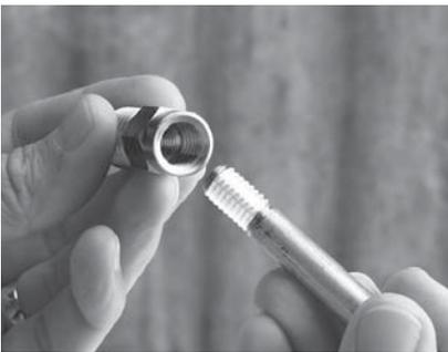
1. For  $1\frac{1}{2}$ " valves with a  $\frac{3}{8}$ " (10mm) thread on the lever first remove the lever lock nut, then apply PTFE tape or an appropriate locking compound to the thread on the lever:
