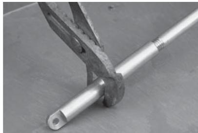
**2.** Screw the arm extension onto the lever using PTFE tape or approved sealant.
