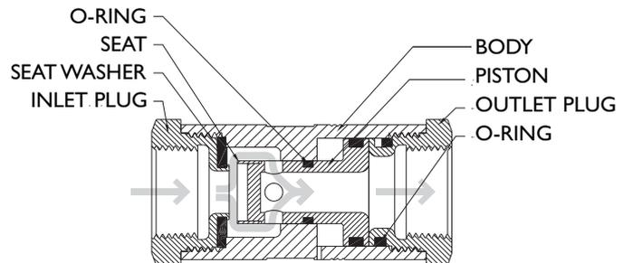
The valve operates on the principle of differing surface areas. In the example of a 2:1 screwed-ratio valve the upstream piston surface area is half that of the downstream surface area. Other ratios are obtained by altering the area relationship of the valve.
