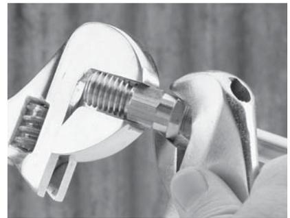
3. For 2" valves with a  $\frac{1}{2}$ " thread on the lever; screw the adaptor on to the thread until tight then tighten the lock nut against the adaptor with a spanner:
