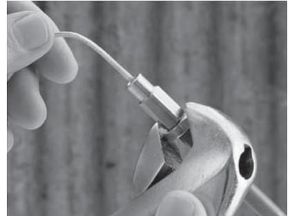
**3.** Where the lever lock nut is fitted, tighten it against the female end of the float attachment cord.
