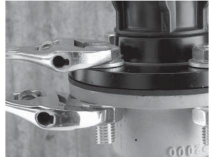
3. Tighten the bolts with a spanner ensuring the bolts are torqued up correctly in an appropriate sequence.
