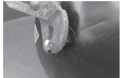
**3.** Screw the float adaptor into the float (ball).
