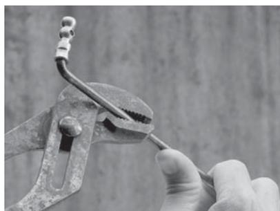
2. By using a pair of multi-grips or equivalent the lever can then be bent to the necessary angle.
