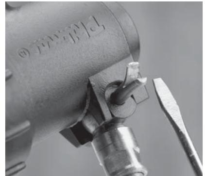
**6.** Adjust the arm and then refit. Once the correct arm angle is achieved ensure the pivot pin tabs are flared outward by using a small screwdriver
