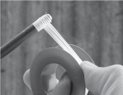
**1.** Where a lever lock nut is not fitted apply a small amount of PTFE tape or an appropriate locking compound to the thread on the lever:
