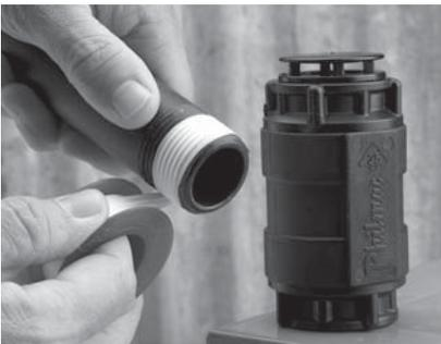
**1.** Apply PTFE tape or approved sealant to the male thread the air relief valve is to be screwed into. Sufficient tape needs to be applied to ensure a watertight seal.
