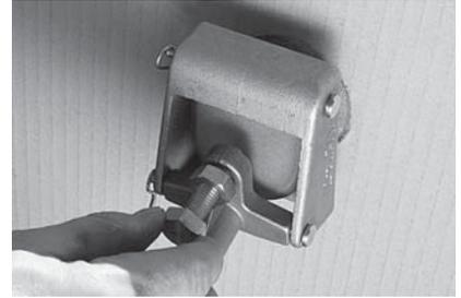
**3.** Adjust the float level by screwing the adjusting bolt in or out of the cam. Screwing the bolt out lifts the water level, screwing it in lowers the water level. Once the correct level is found ensure the nut is tightened to stop the adjusting bolt from moving.
