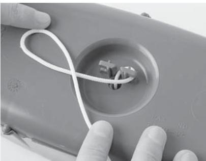
1. Insert the cord through bottom hole of the float, ensure the top of the float is BELOW the rim of the trough then place the cord around the right hand lug. Make a loop.
