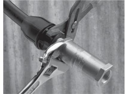
3. Using a pipe wrench or multigrips on the hex end of the valve, screw it into the male thread until tight. Where necessary ensure the male thread is held stationary to avoid it from moving.
