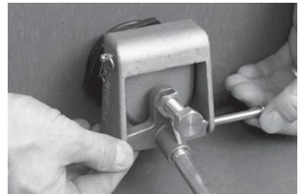
**5.** Re-attach the lever arm assembly to the body by re-inserting the clevis pin and fitting the cotter pin. Adjust the float level by screwing the adjusting bolt in or out of the cam as per the top installation.
