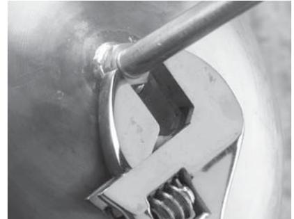
3. For 2" valves tighten the nut against the copper float (ball) to lock it in place.
