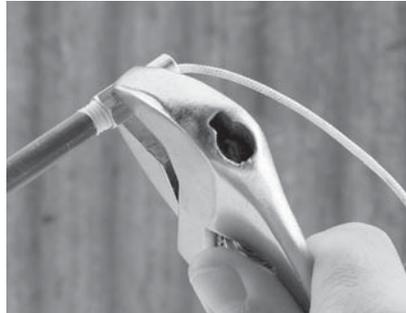
**2.** Screw the female end of the float attachment cord into the lever and tighten up using a spanner or equivalent.
