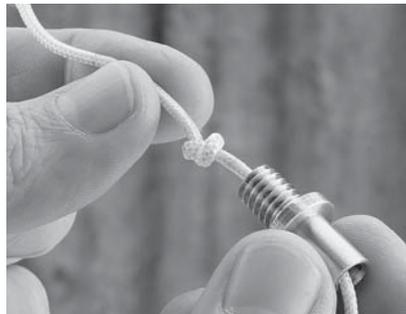
**5.** Check the float is at the correct level. If not, pull the cord through the female and re-do the knot making the cord shorter in length.
