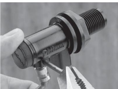
1. Where necessary bend the lever arm to adjust the water level. This can be done by removing the lever arm assembly by first straightening the tabs on the end of the pivot pin with a pair of pliers then slide it out.
