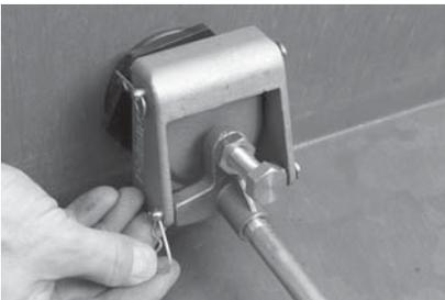
**1.** Remove the clevis pin and slide the cotter pin out from the cam/arm assembly.
