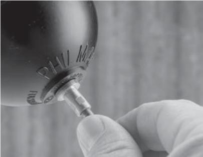
1. Thread the float (ball) onto the lever arm of  $\frac{3}{8}$ " and  $\frac{1}{2}$ " valves and tighten fully to the flange on the adaptor:
