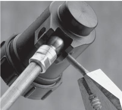
**4.** Where necessary bend the lever arm to adjust the water level. This can be done by removing the lever arm assembly by first straightening the tabs on the end of the pivot pin with a pair of pliers then slide it out.
