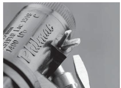
3. Adjust the lever arm and then refit. Once the correct lever arm angle is achieved ensure the pivot pin tabs are flared outward by using a small screwdriver.
