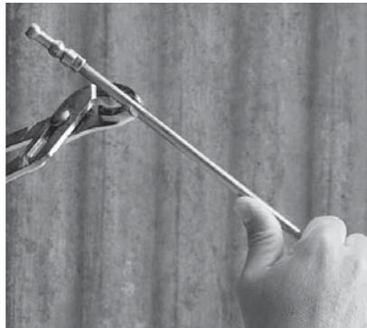
**5.** By using a pair of multi-grips or equivalent the lever can then be bent to the necessary angle.
