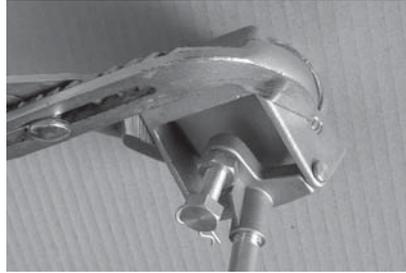
**2.** Tighten the body using a pair of multigrips or a spanner. Ensure the body is in an upright position so that the lever arm moves in a vertical direction.
