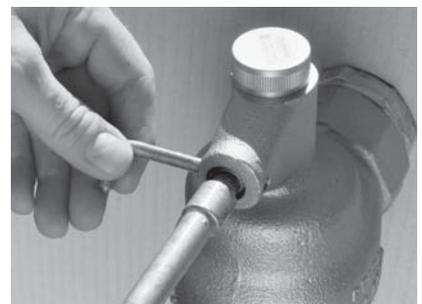
**6.** Remove the pivot pin from the body and fit the lever arm then ensure the pivot pin tabs are flared outward by using a small screwdriver:
