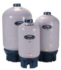
Best of all, these tanks will never rust — they're mounted on a moulded base, and are constructed from 3 miles of glass-reinforced plastic that is wound into epoxy resin strand by strand in a Sta-Rite proprietary pattern that maximises strength. We recommend these tanks where water quality causes corrosion problems. Another benefit of this construction is that they are around half the weight of comparable steel tanks — making installation by one person a reality.
