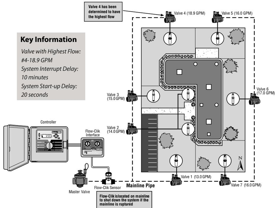
**Lateral Line Break:** If a break should occur on zone #3, the Flow-Clik would sense a "high flow" condition (>21 GPM) and would shut down the system for the prescribed interrupt period.
